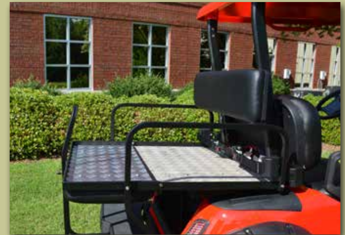
Rear flip seat: diamond-plated aluminum, 350 lb load capacity
